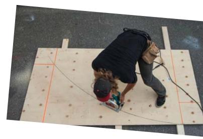
Once you've cut your first transition, remove the first piece of plywood and use it as a template for your second transition. Trace your second transition then move the first transition out of the way. Now, using the same process, cut your second transition. You will have an oblong surf board piece of wood left over. You can use this offcut to create a "Wood Scrap Art project" listed in this manual! Set aside.
