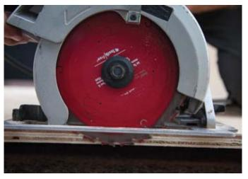
• Use your hand to manually hold up the guard and start cutting your transition. Start by drop cutting through the place where the platform and ramp meet
