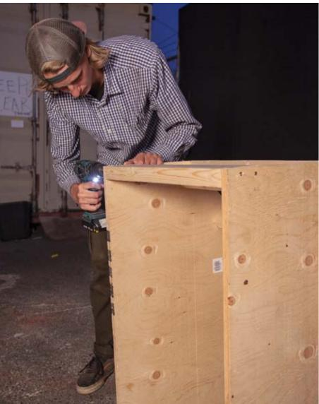
Go back and add a second screw on all the ribs, on both sides of the transition and the supporting ribs, double checking that each rib is flush.
